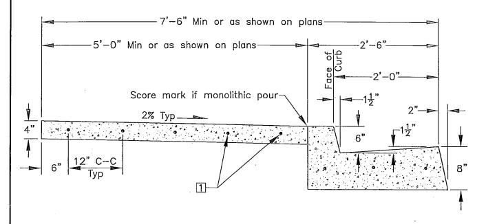
VERTICAL CURB, GUTTER AND SIDEWALK
